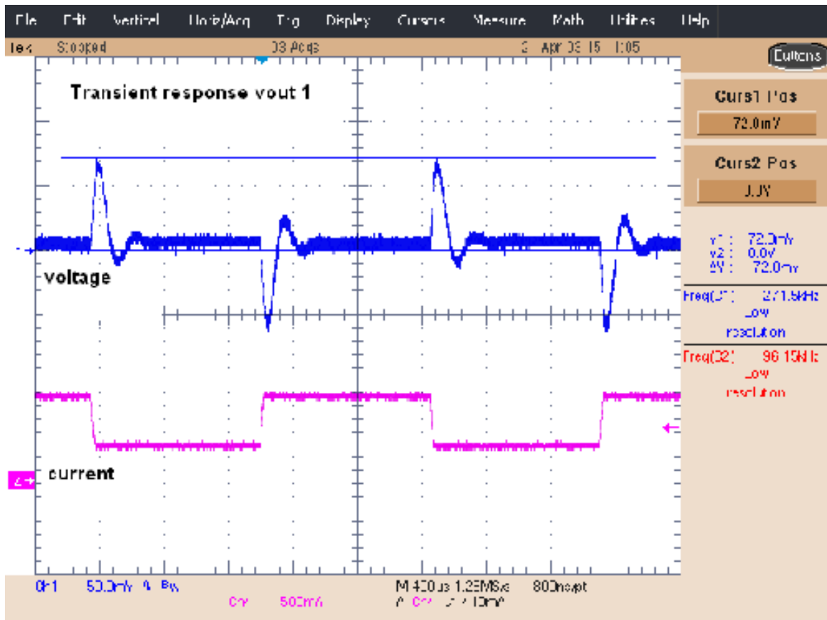
FIGURE 6. Transient Response Vout1
